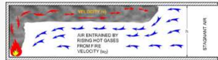
Fig. 2: The advance of the leading edge (or "nose") of a buoyant layer of hot gases
